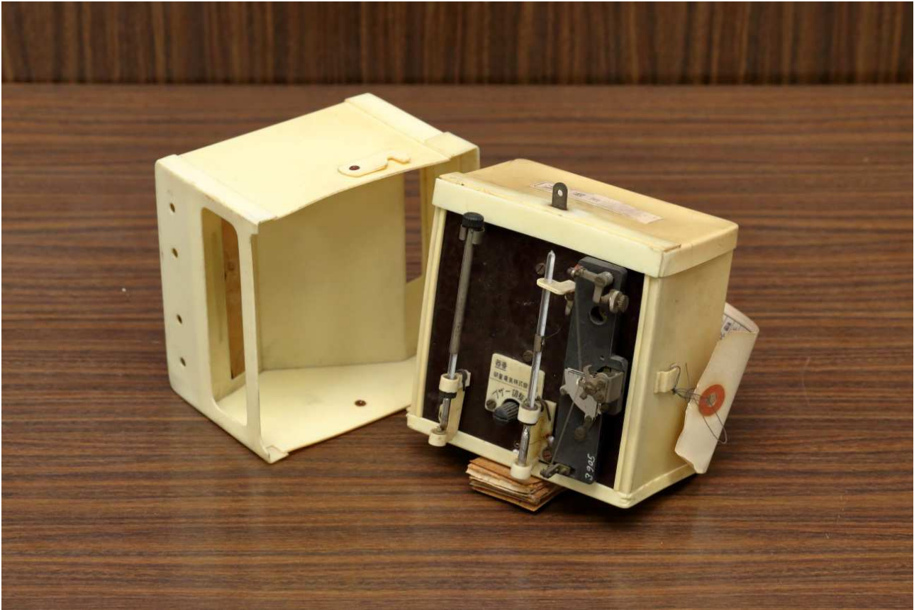
Figure 1.2: Photograph of the 3-SHIKI ON-SHITSU HASSHINKI (also called as S43 type radiosonde). This radiosonde was manufactured by the Meisei Electric Co., LTD for the Imperial Japanese Army. The Japan Meteorological Agency (JMA) employed this radiosonde from the Imperial Japanese Army after the World War II, and used it until the new S48 type radiosonde was developed in 1949.
