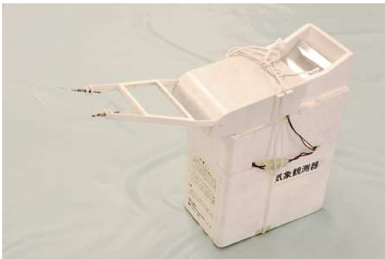
Figure 1.6: Photograph of the RS2-80 type rawinsonde. This type uses the frequency modulation method for the data transmission, and is equipped with a thermistor thermometer and carbon hygrometer.
