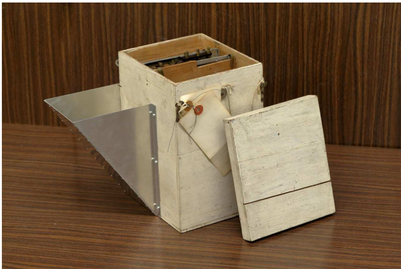
Figure 1.3: Photograph of the S48 type radiosonde. Data were converted to the Morse coded data, and sent by the fixed 27.7 MHz carrier frequency.
