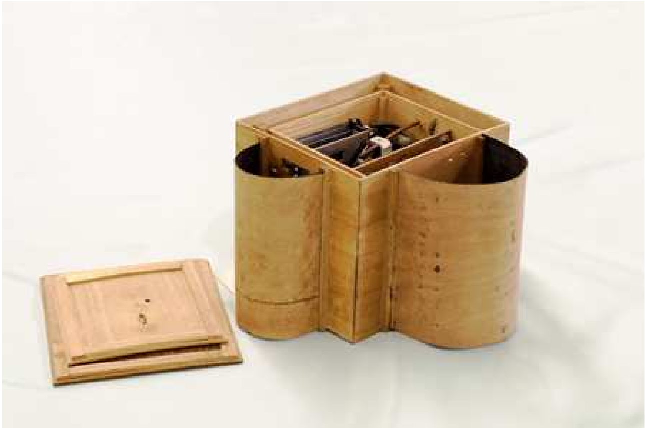
Figure 1.1: Photograph of the Central Meteorological Observatory Type No.1 radiosonde (also called as S38 type radiosonde). This radiosonde is composed of a pressure instrument part, temperature instrument part and humidity instrument part. Each part is composed of a sensor and transmitter. This photograph shows a later version (1942- ) of the S38 type radiosonde, for the paulownia wood was used for the radiosonde housing.
