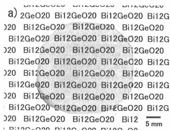
Fig. 3. \text{Bi}_{12}\text{GeO}_{20} single crystal grown by the pulling-down method.
