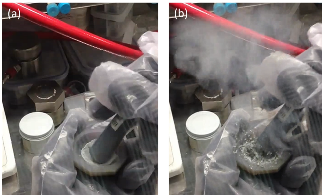
Fig. 3-4 Images of hand-mixing AB with \text{LiAlH}_4 in an argon glovebox; (a) in the beginning of the hand-mixing (before eruption), (b) After 120 seconds (gas eruption occurs.).
