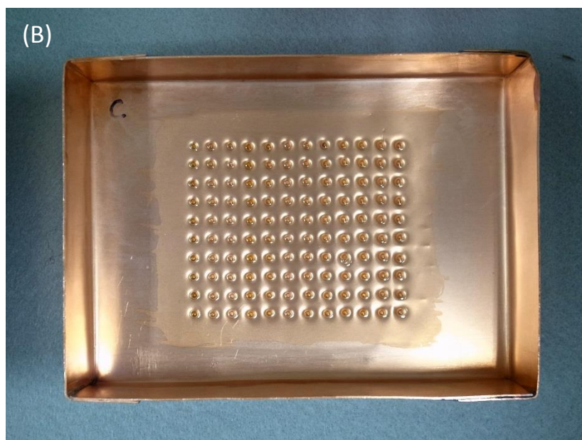
Fig. 2-1. The droplet freezing assay system (A) and copper plate used in this assay (B). Mineral oil was pasted on the surface of the dimples on the copper and sample droplets (2 \mu L) were loaded on the dimples. This copper plate was cooled by programmable freezer and number of frozen droplets were counted. Freezing temperature of 50% of samples was determined as FT 50 .
