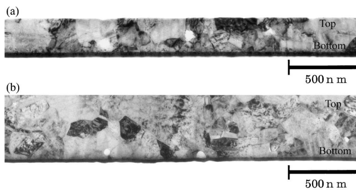
Fig. 3.25 Average grain size distribution of 80-nm-wide and 500-nm-high Cu interconnects after annealing at 400 °C for 0.5 h. The grain size increased with the distance from bottom of trench.
