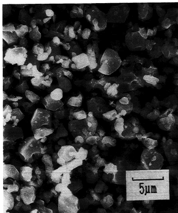
Fig. 3 Scanning electron micrograph of \text{Al}_3\text{Ti} powders reduced by \text{CaH}_2 for 10.8 ks at 1273 K. The molar ratio of Al:Ti in the starting oxide mixture was 85:15.
