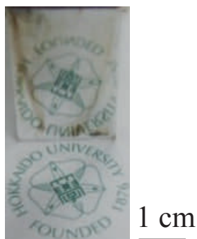
Fig. 7 Photograph of the Al electroplating on Cu plate using Al mesh counter electrode in EMIC- \text{AlCl}_3 ionic liquid containing 20 \text{ mmol L}^{-1} Phen at 60^\circ\text{C} with no stirring.
