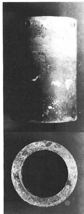
Fig. 8 Appearance of \text{TiB}_2/\text{TiN} coated steel after thermal cycle test of 2500 times. The photograph was taken after chemical removing of aluminum adhered to sample.
