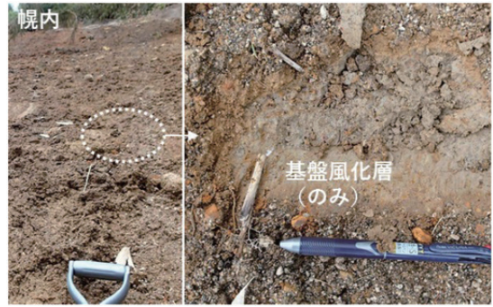
図-5 基盤風化層型の滑り面 Fig.5 Slip surface on the weathered bedrock
