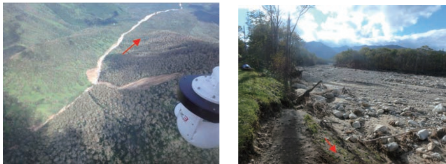
写真-13 久山川で発生した土石流 (左 源頭部の崩壊と土石流, 右 清水町旭山地区付近での土石流流下状況) Photo 13 Debris flow at Kyusan river (Left : Shallow slope failure and debris flow, Right : Debris flow at Asahiyama, Shimizu Town)
