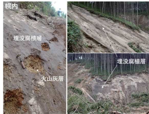
図-6 埋没腐植層型の滑り面 Fig.6 Slip surface on the buried humus layer
