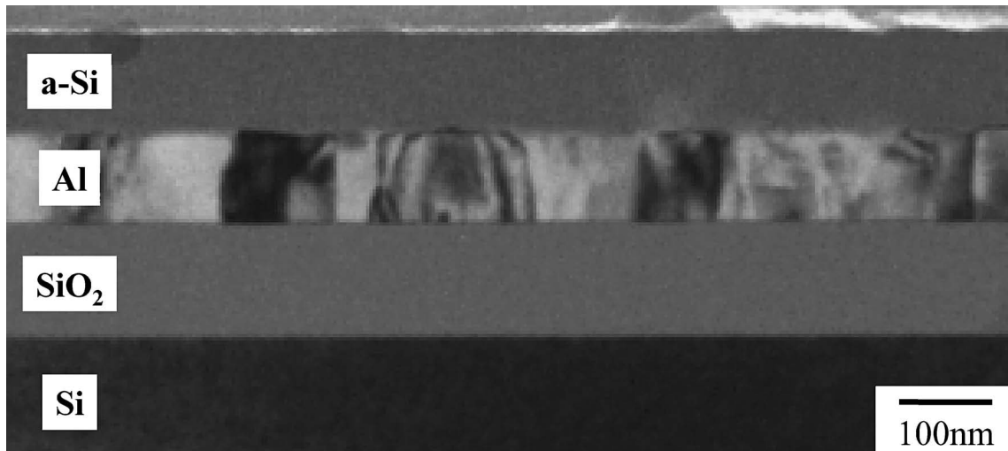
Fig. 1 Cross-sectional BF-TEM image of as-deposited a-Si/Al film.
