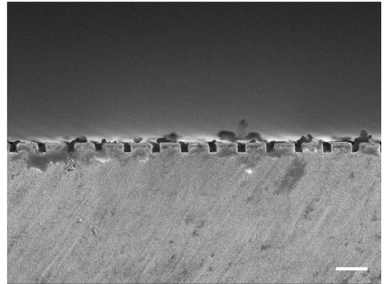
Figure 7. A photo of the micro- and nanofluidic device and SEM images of nanofluidic channels fabricated by the electron beam lithography technique; scale bar, 1 \mu\text{m} .
