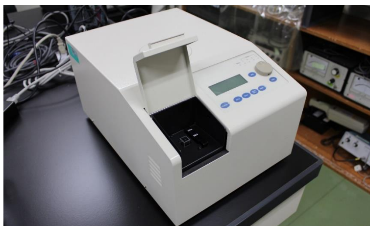
Figure 2.2 Photo of a conventional commercial fluorescence polarization (FP) apparatus (FP-715, JASCO Co., Tokyo, Japan). A cuvette is used as the sample cell and the number of samples is limited to one for each measurement.
