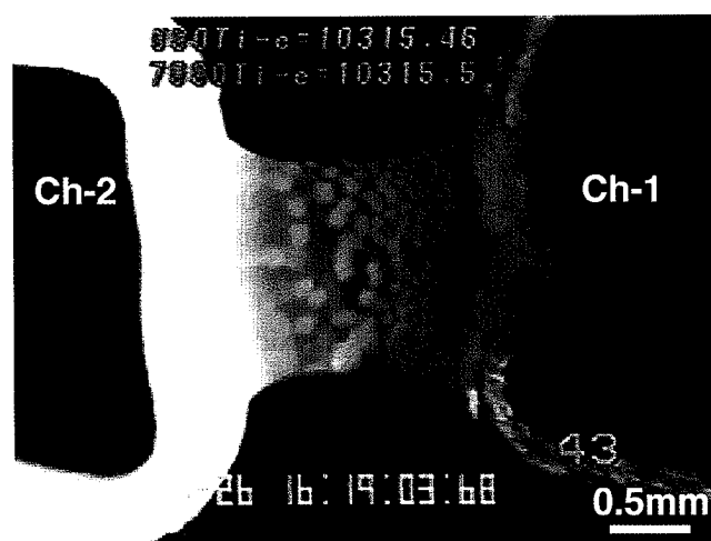
Fig. 13. Crystallization behavior of a simulated mold slag when Ch-1 was cooled with 50°C/s. (5% Na 2 O, 6.8% Al 2 O 3 , C/S=1)
