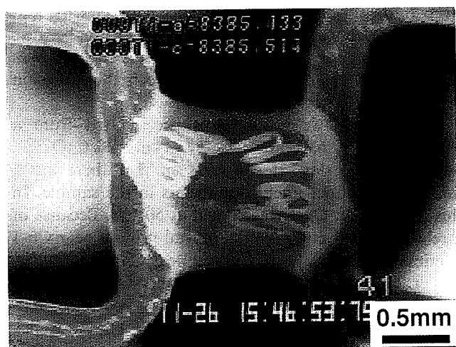
Fig. 10. Result of in situ observation by DHTT of a simulated mold slag at 1550°C. (5% Na 2 O, 6.8% Al 2 O 3 , C/S=1)
