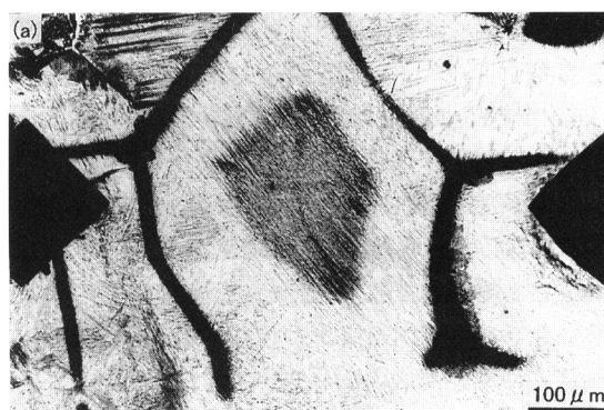
Fig. 5. Microstructure of fine columnar \gamma grain region.
