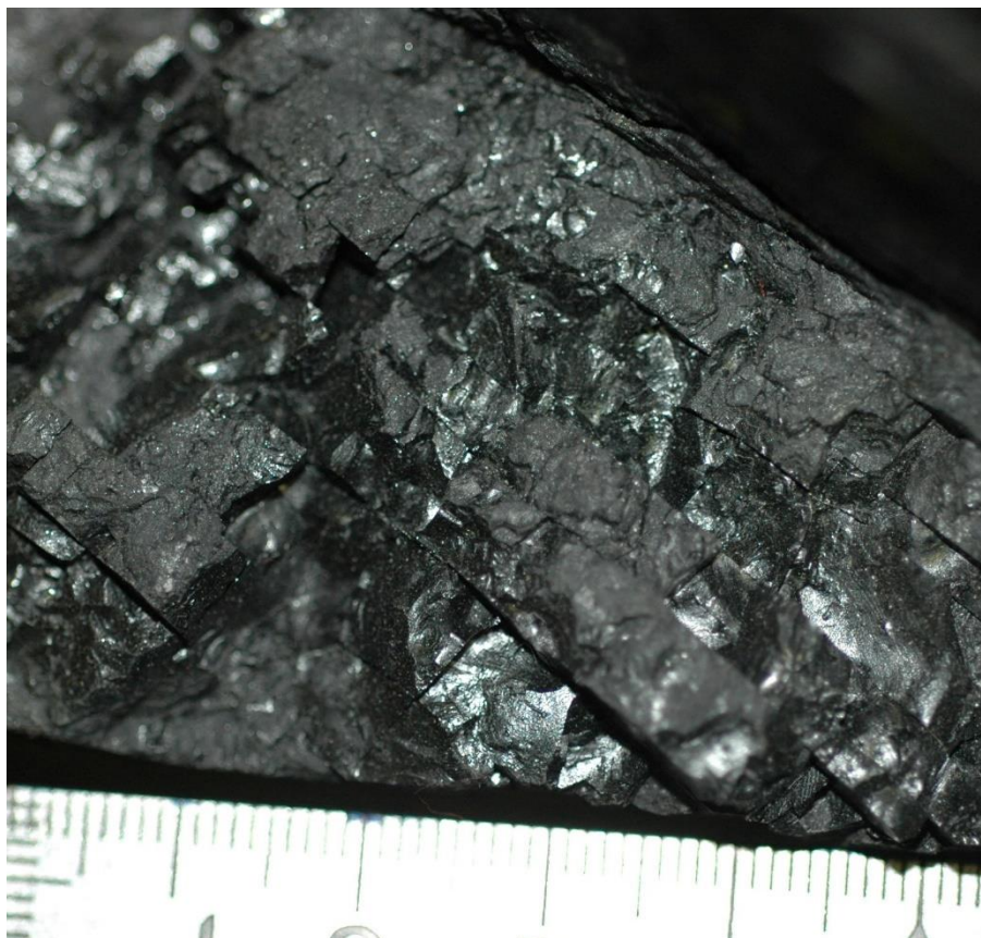
Fig.3.1 Picture of the bedding plane of the coal block.
