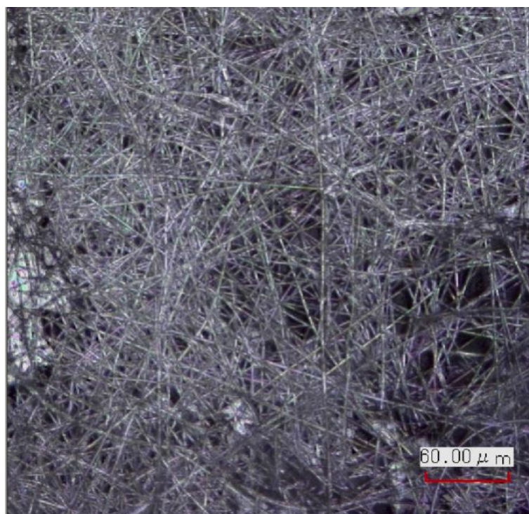
Figure 3-8 Fiber morphology after mixed solvent DMF/EtOH (1/1, w/w) treatment on PU sheet.
