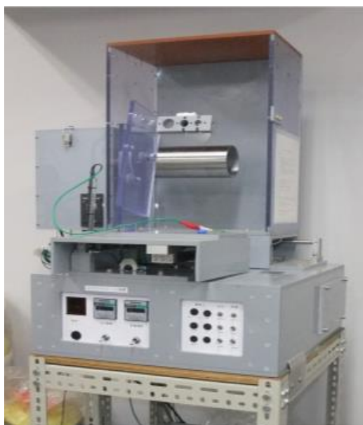
Figure 3-2 An electrospinning setup view
