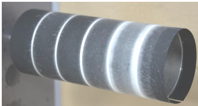
Figure 3-7 PU sheet placed on collector plate with double side tape
