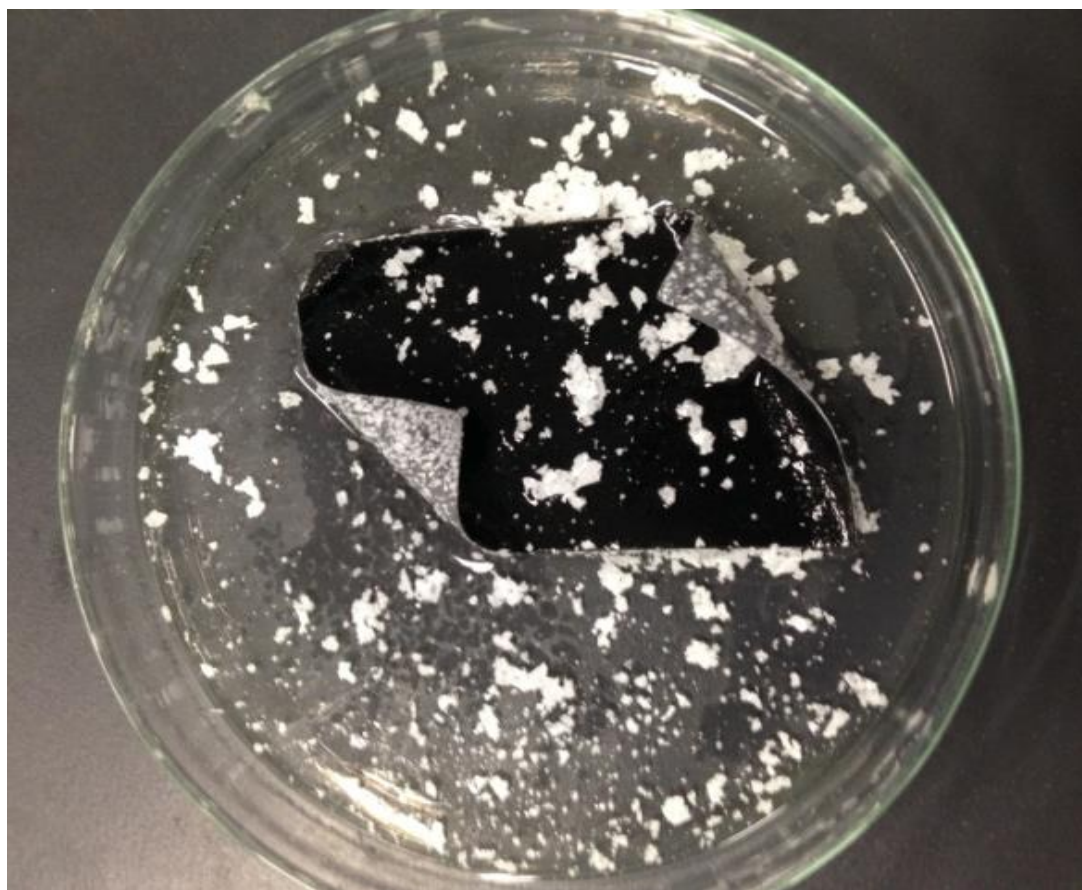
Figure 3-13 PU sheet morphology in oven under 3 days at 60 °C.
