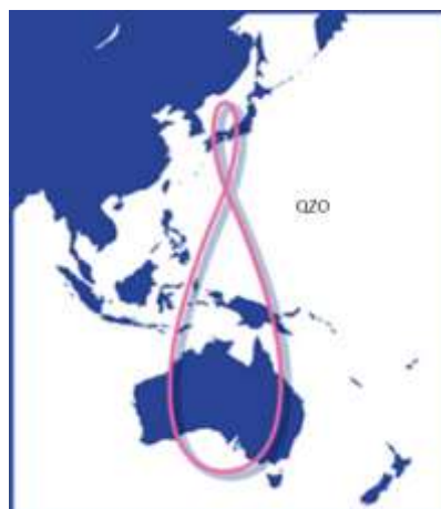
Fig. 2. 3. Coverage of QZSS and its trajectory (Cabinet Office, 2017a).
