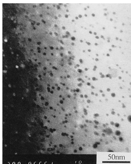
Fig. 13. Transmission electron micrograph of oxide particles in Mm13 cladding.
