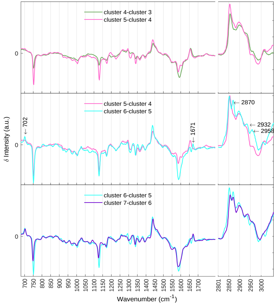
Figure 4.12: The superimposed plot of mean difference spectra of 5 adjacent spectral clusters (cluster 3 (red) to cluster 5 (purple))
