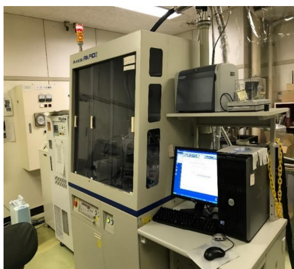
Figure 2.6. XRD machine Rigaku Max-007 HF in Okayama University.
