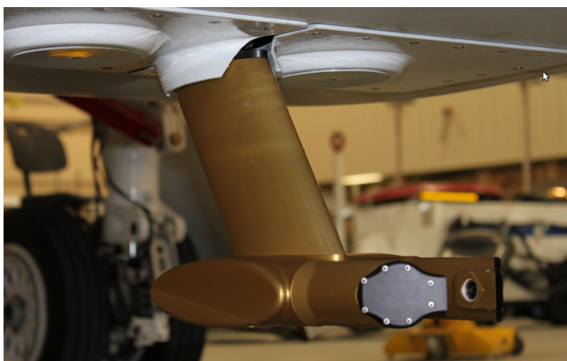
Figure 2.1: Fast Cloud Droplet Probe (FCDP) for measurement of the number concentration and size of ice particles. Laser spectrometer mounted on the tip of the arm (center of the picture) measures the forward Mie scattering from ice particles. Taken from https://espo.nasa.gov/home/sites/default/files/images/IMG_0772.JPG .
