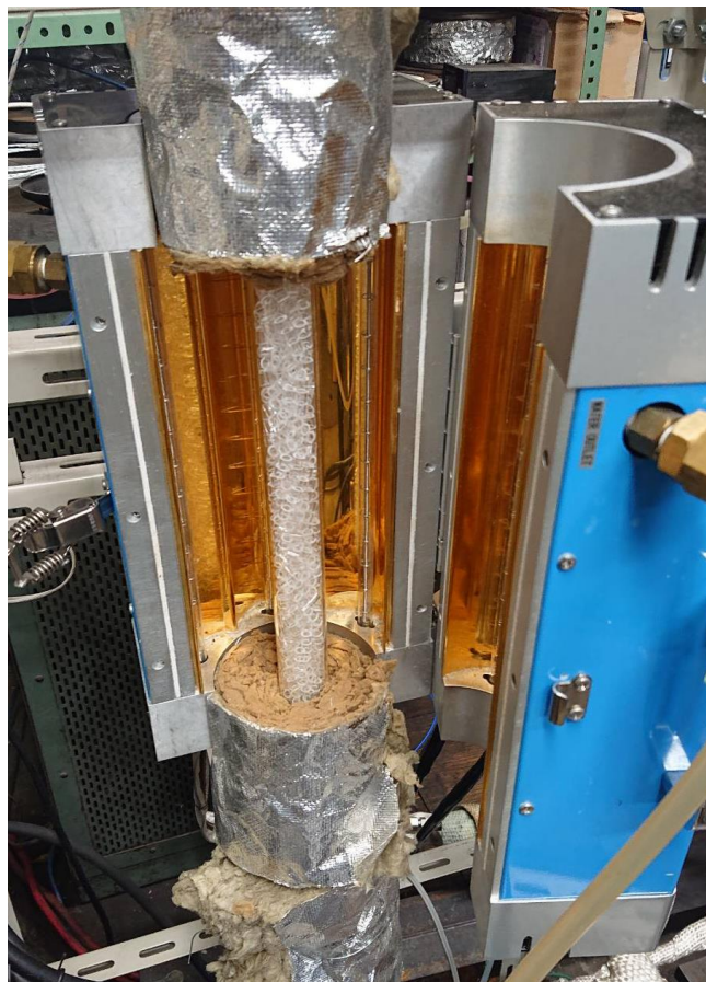
Fig. 2.6 Gold image furnace and quartz tube.
