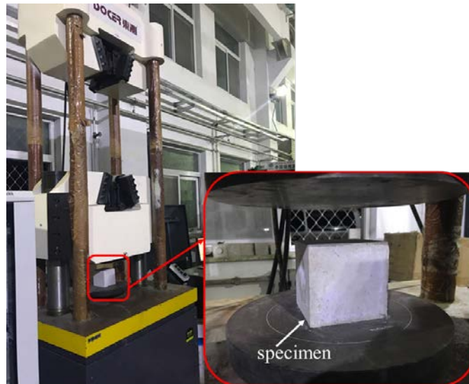
Fig. 1. The set-up of the compressive test
