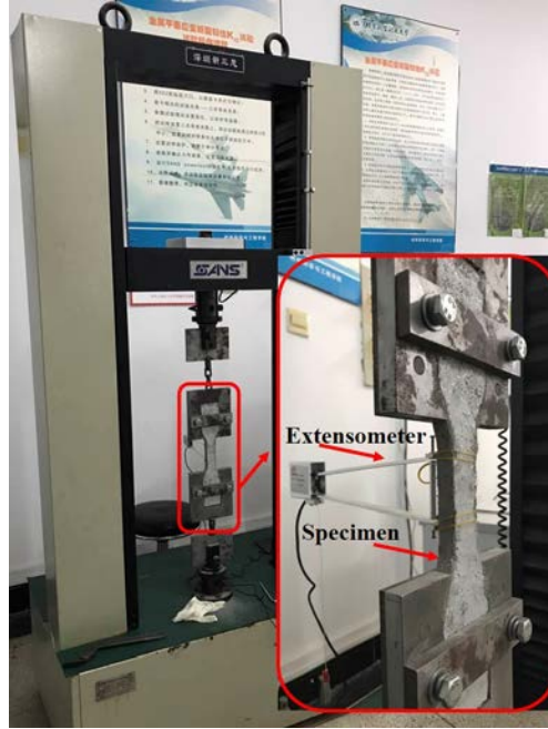
Fig. 2. The set-up of the tensile test
