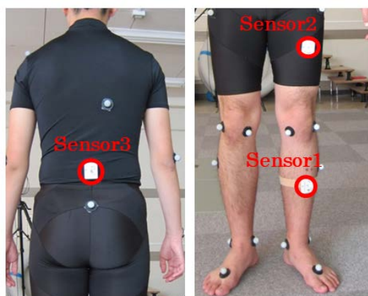
Fig. 5.2: Arrangement of inertial sensors
