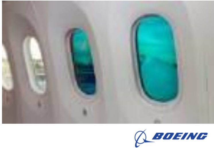
Figure 6. Electrochromic windows used on Boeing 787 aircraft.
