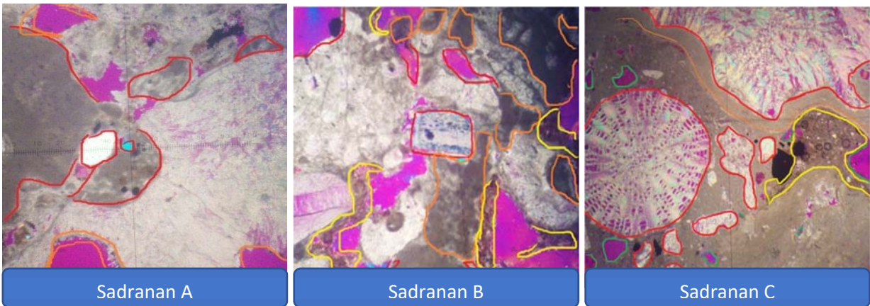
Figure 6. Sadranan beachrock cement vision using 100x (yellow pattern represented grain matrix and orange pattern represented cement).
