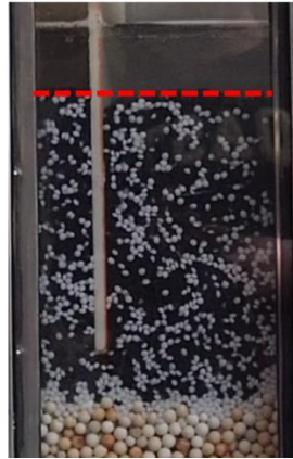
Figure 6-11. Photographs of batch-type jig experiment of ABS/POM at L/H ratio of 65:35 with a vertical restraining wall; (a) before and (b) after jigging.
