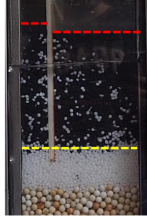
Figure 6-11. Photographs of batch-type jig experiment of ABS/POM at L/H ratio of 65:35 with a vertical restraining wall; (a) before and (b) after jigging.
