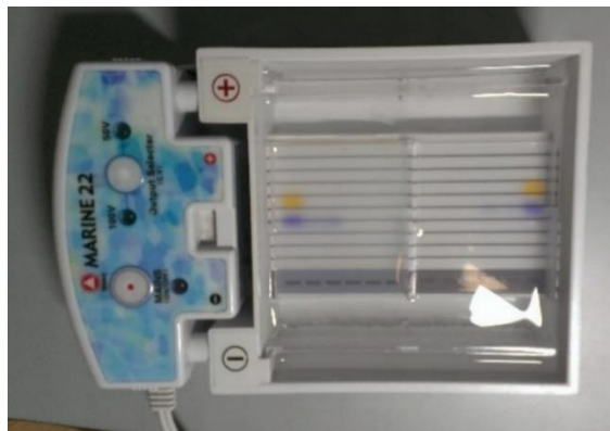
Fig. 5.5: Horizontal gel electrophoresis equipment
