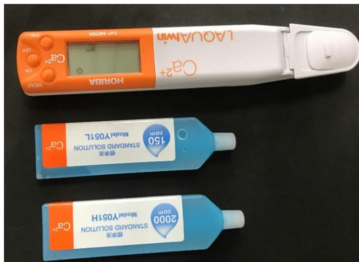
Fig. 2.2: Calcium ion meter with standard solutions for calibration
