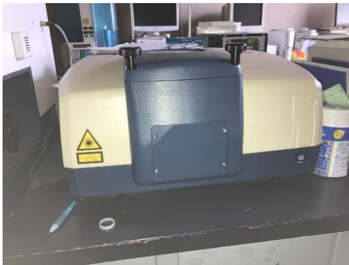
Fig. 5.11: FTIR spectrometer with an attenuated total reflectance (ATR) attachment
