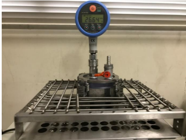
Fig. 2.5: Calcimetric meter setup
