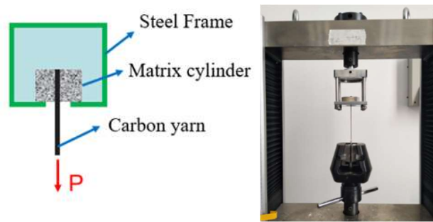
Fig. 2.1 Test setup for pullout tests
