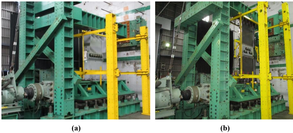
Fig. 5.1.2 Experimental setup for full-scale tests: (a) Specimen S-1 and (b) Specimen S-2 1)
