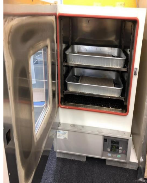
(b) Drying process in the oven at temperature of 120 °C
