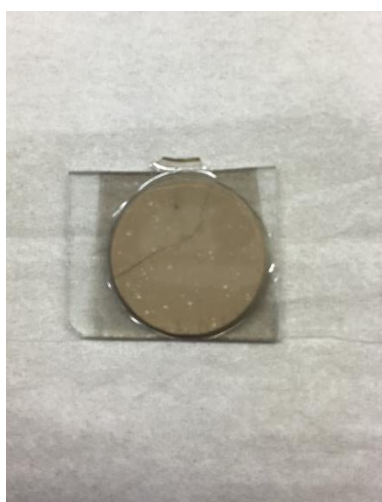
Figure 3-10 Thin sectioned polished sample surfaces with Pt coating
