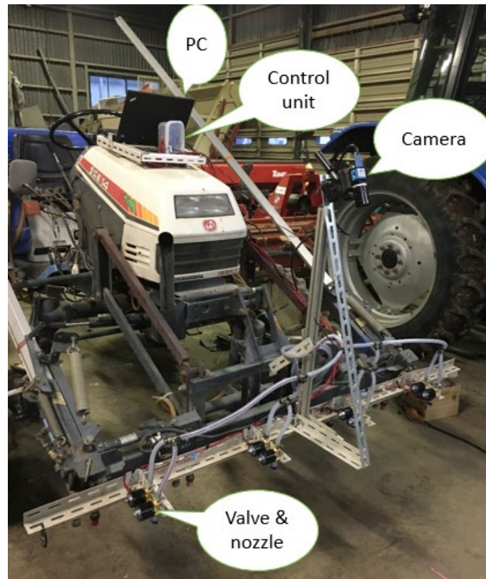
Fig. 36 The experiment setup of sprayer system into Iseki machine.
