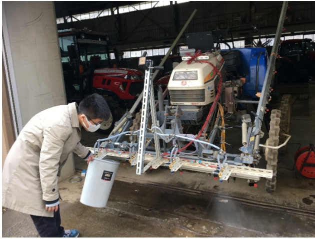
Fig. 39 The calibration of volume of each sprayer.
