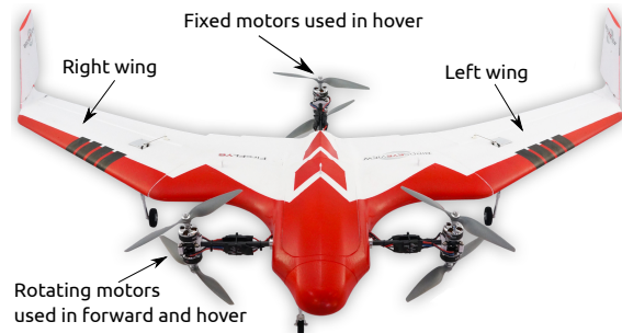
Figure 4: Vertical Take-Off and Landing UAV “Firefly6” (wingspan 1520 mm). The forward axis supports four motors, which can rotate by 90° for flight transition between a hexacopter and a fixed-wing.
