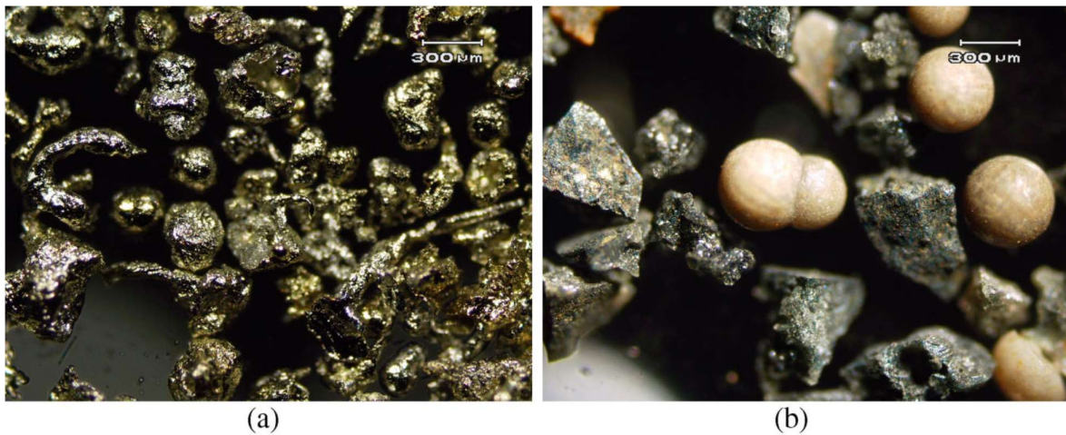
Fig 2.2. (a) Optical micrograph of tin debris from MISTEE test and (b) optical micrograph of PREMIX 18 debris showing angular and spherical pieces. (Tyrprekl et al. 2014)
