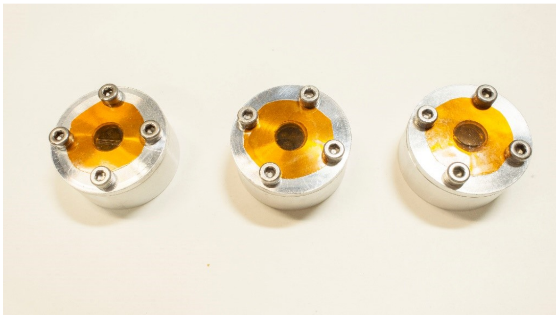
Figure 5.1 Home-made sample holders.
