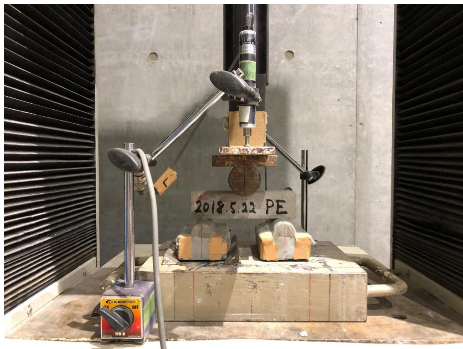
Figure 2.12 Flexural strength tests for PCM specimens.
