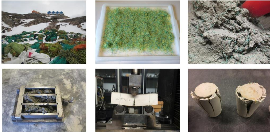
Figure 1.11 Recycled HDPE fiber from waste fishing nets.
