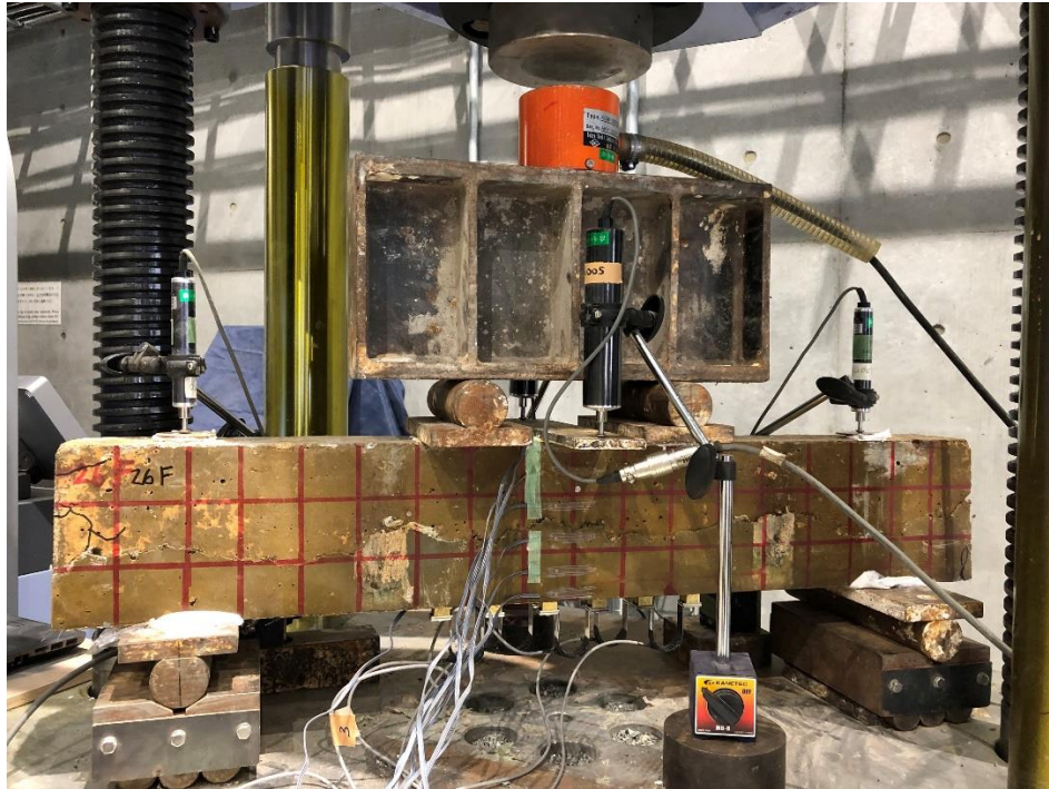
Figure 2.11 Four-point flexural test for RC beams.
