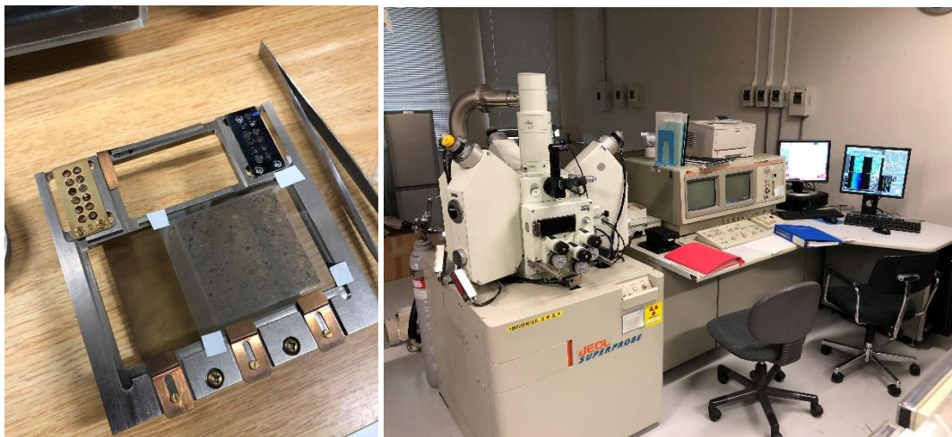
Figure 5.6 (Left) Testing sample on sample stage and (Right) EPMA device.
