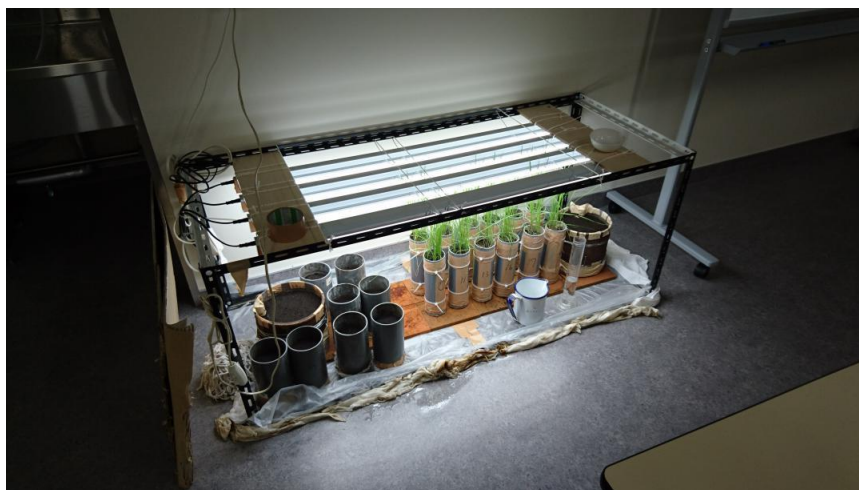
Figure 7.4 Example of grassed soil specimens in growth room.
