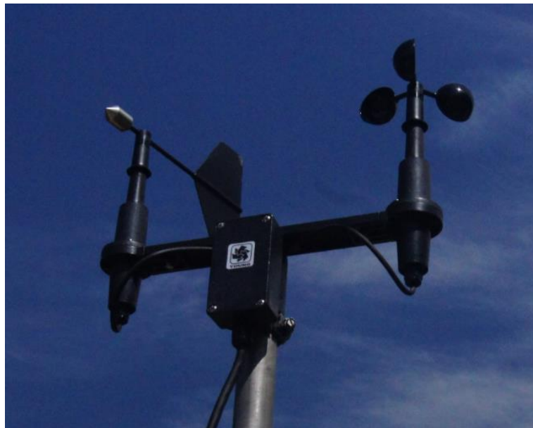
Figure 3.7 Wind speed and wind direction sensors.
