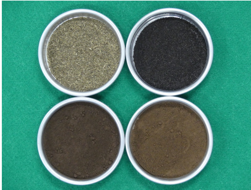
Fig. 3.9 Appearances of raw dairy manure (top left), the manure prepared at 0.1 MPa (top right), 0.3 MPa (bottom left), and 1.0 MPa (bottom right). All samples were dried before photographs were taken to eliminate the effect of water on the color.
