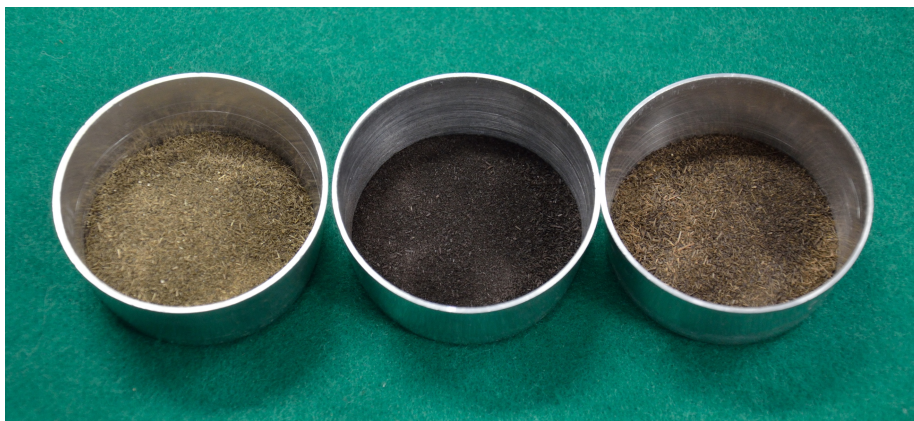
Fig. 2.4 Appearance of raw dairy manure (left), the manure prepared under air at 90 °C (center), and the manure treated under N 2 at 90 °C (right). All samples were dried before photographs were taken to eliminate the effect of water on the color.
