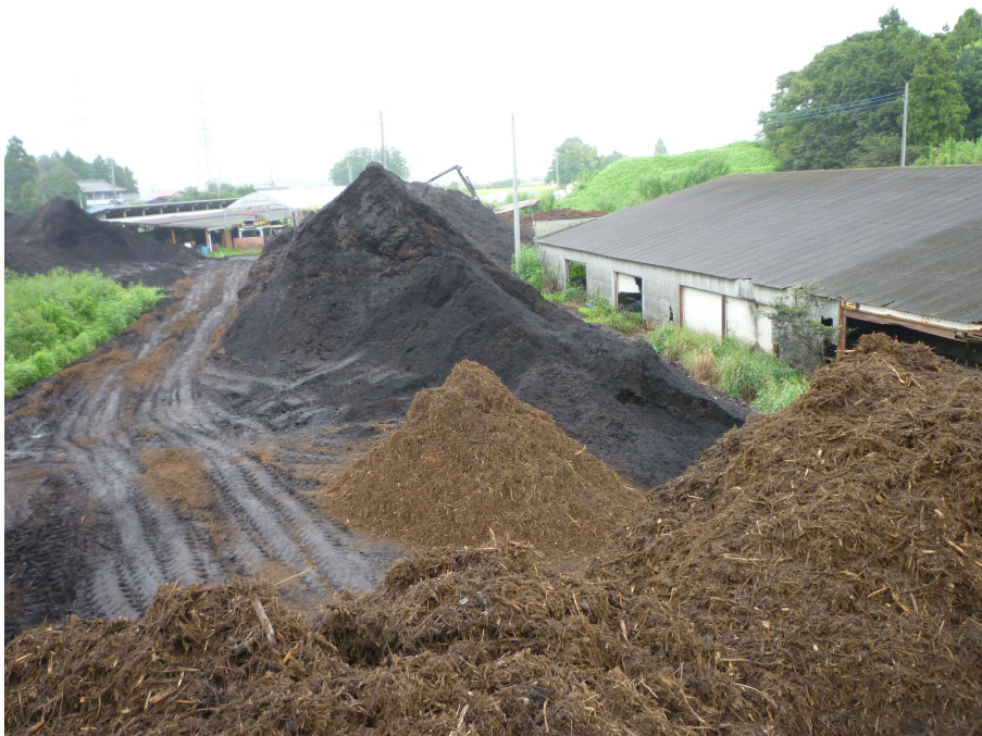
Fig. 2.1 A picture of the wood chip deposition site. Fresh wood chips (near side pile) were converted into char-like materials (far side pile) naturally over several months.
