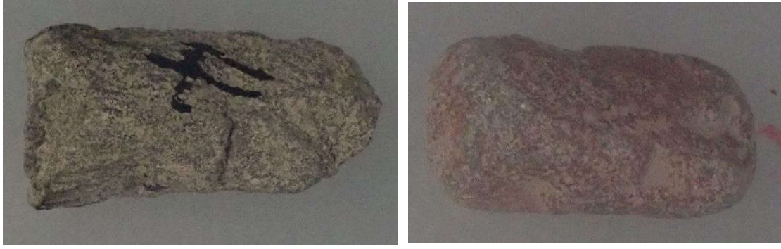
Figure 3-6 Fresh and aged ballast particles before and after LAA test: (a) ballast particle of L0; (b) ballast particle of L60.
