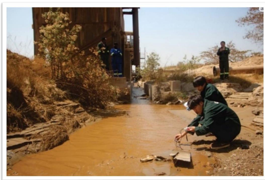
Figure 3. 4. (a) Field measurements of pH, EC and ORP in drainage effluents
