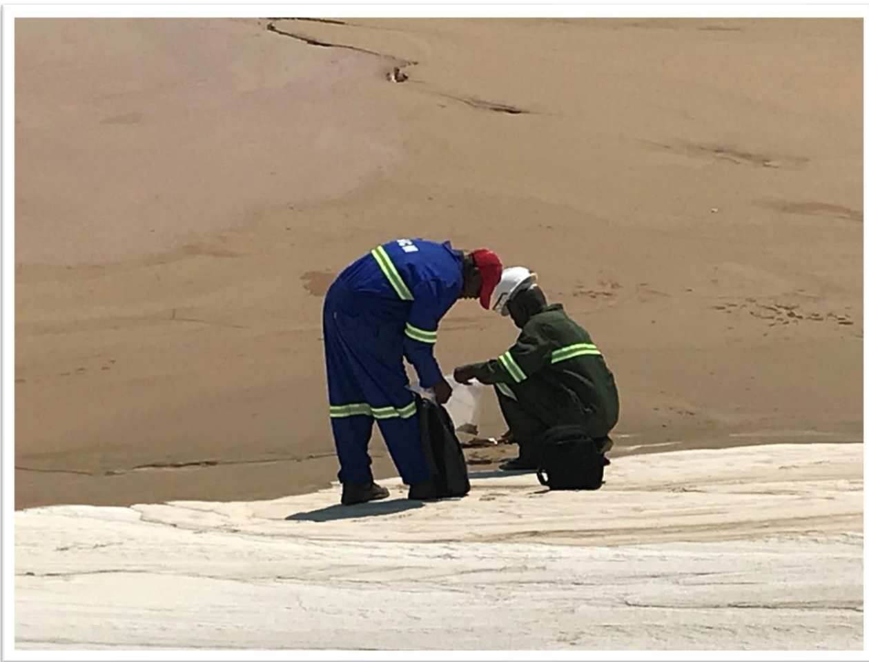
Figure 3.5. Field sampling of solid material at storage sites
