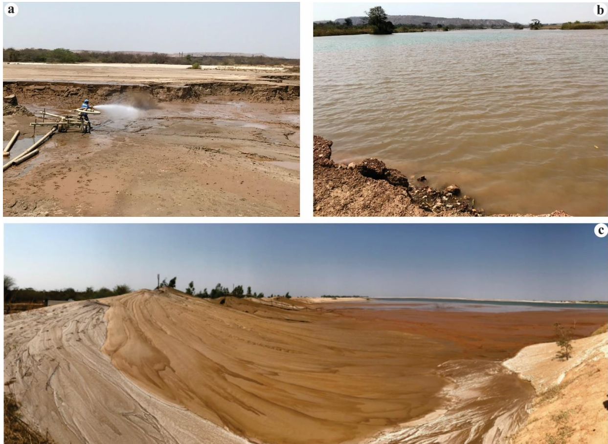
Figure 2. 2. (a) Sedimentation pond; (b) supernatant after sedimentation process; (c) waste heaps
