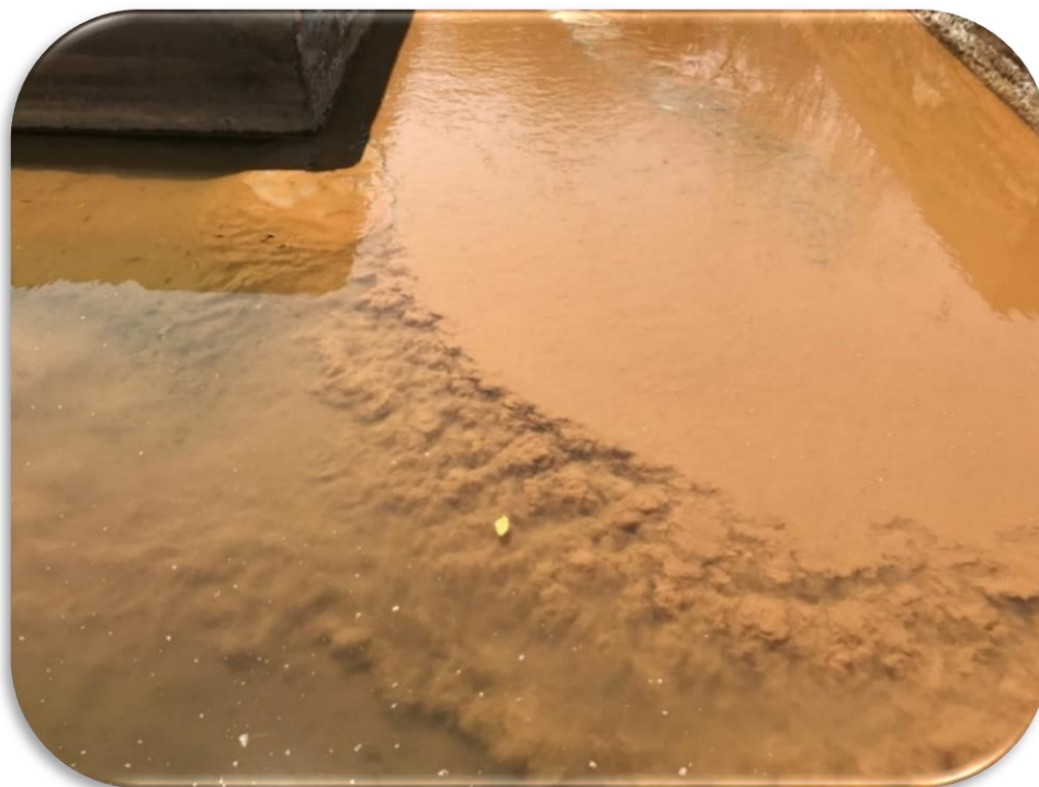
Figure 2. 1. Sludge effluents in mine drainages undergoing sedimentation and settling
