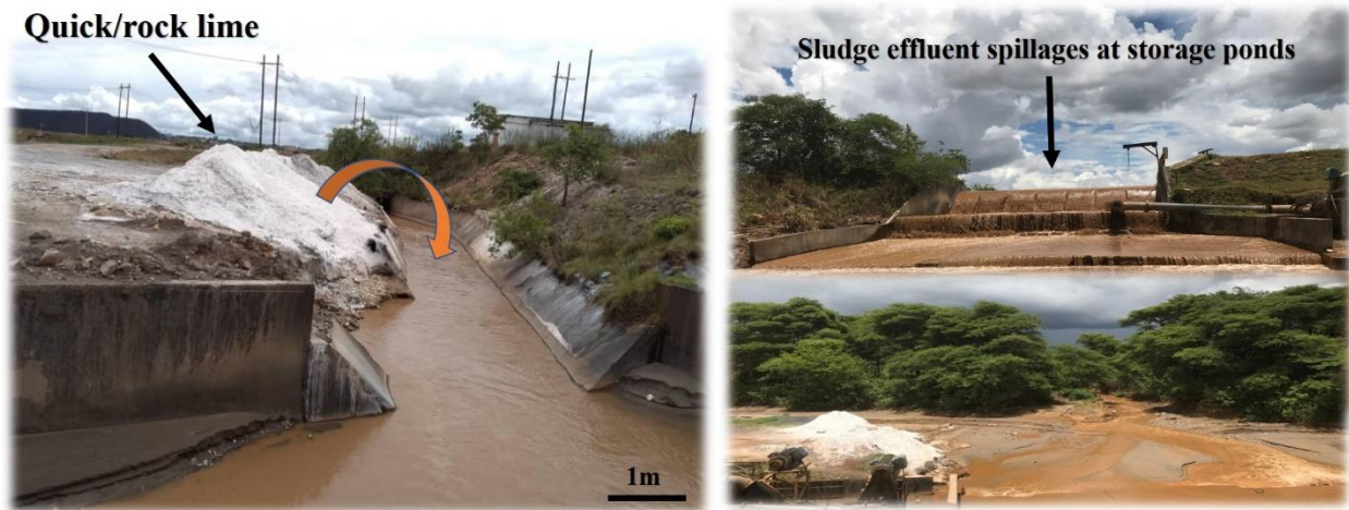
Fig.1.2. a) Un-mechanised lime treatment of mine drainage; b) sludge spillages at storage site
