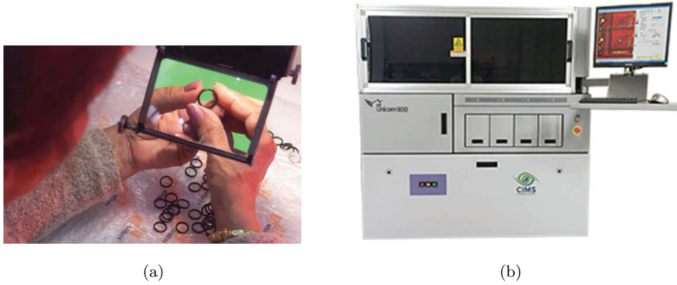
Figure 1.2: Two methods of product defect inspection. (a) Manual inspection [3] and (b) automatic inspection [4]
