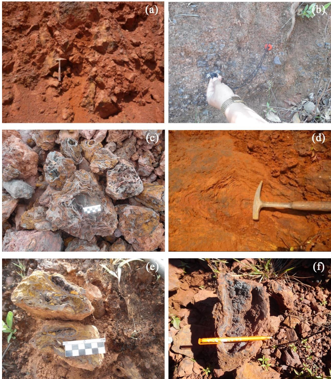
Fig 2.8. Photograph showing a poor bedded nature of limonitic outcrop (a), magnetite grain in weathered limonite outcrop (b), cavernous structure of limonitic ores (c), yellowish-brown colored iron rose texture of limonite ore (d), botryoidal nature of limonite ores (e, f).
