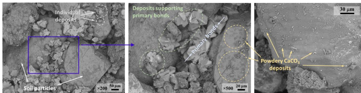
Figure 5.13: Illustration of types of crystallizations formed in MICP treated soil
