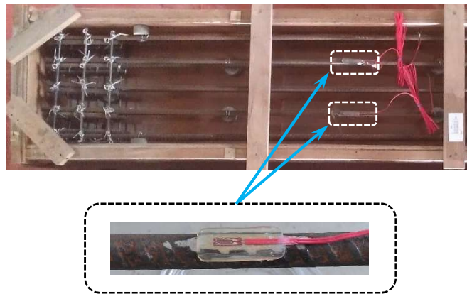
Figure 5: Strain gauges on longitudinal steel.
