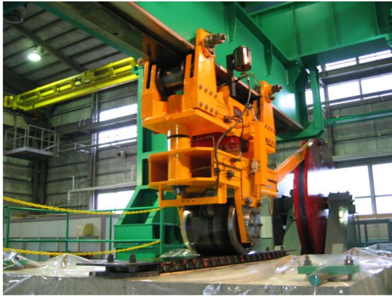
(a) Experimental set-up for cyclic moving wheel loads
