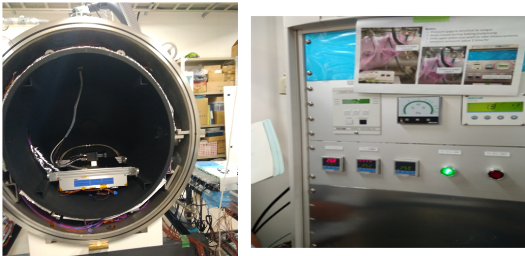
Figure. 3.6. TIS camera is tested in vacuum chamber
