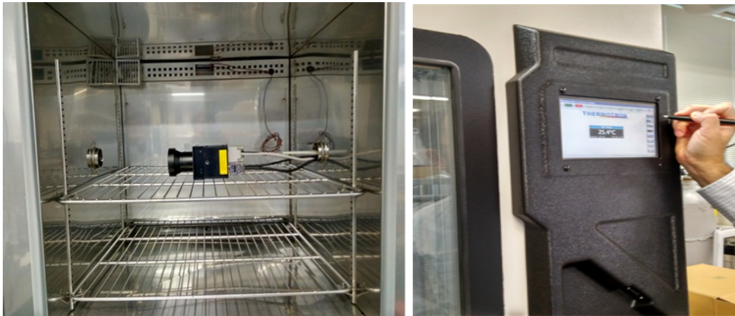
Figure. 3.4. TIS camera inside thermal chamber during thermal test in SMC
