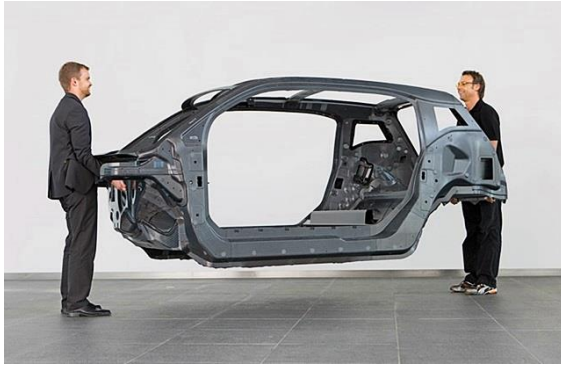
Figure 8. Monocoque body of BMW i3, [23]
