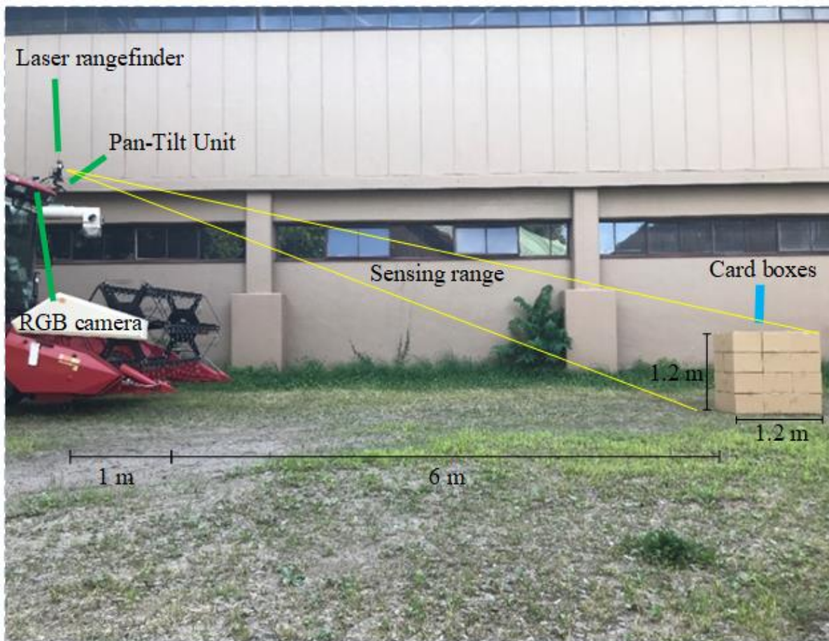
Figure 3.1 Simulation experiment to detect the edge of box.
