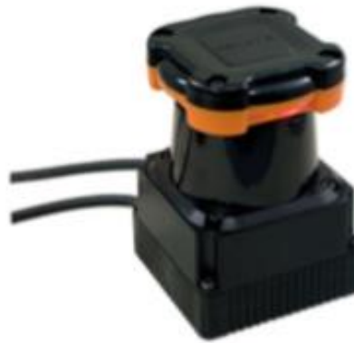
Figure 2.4 Hokuyo UTM-30LX 2D laser rangefinder.
