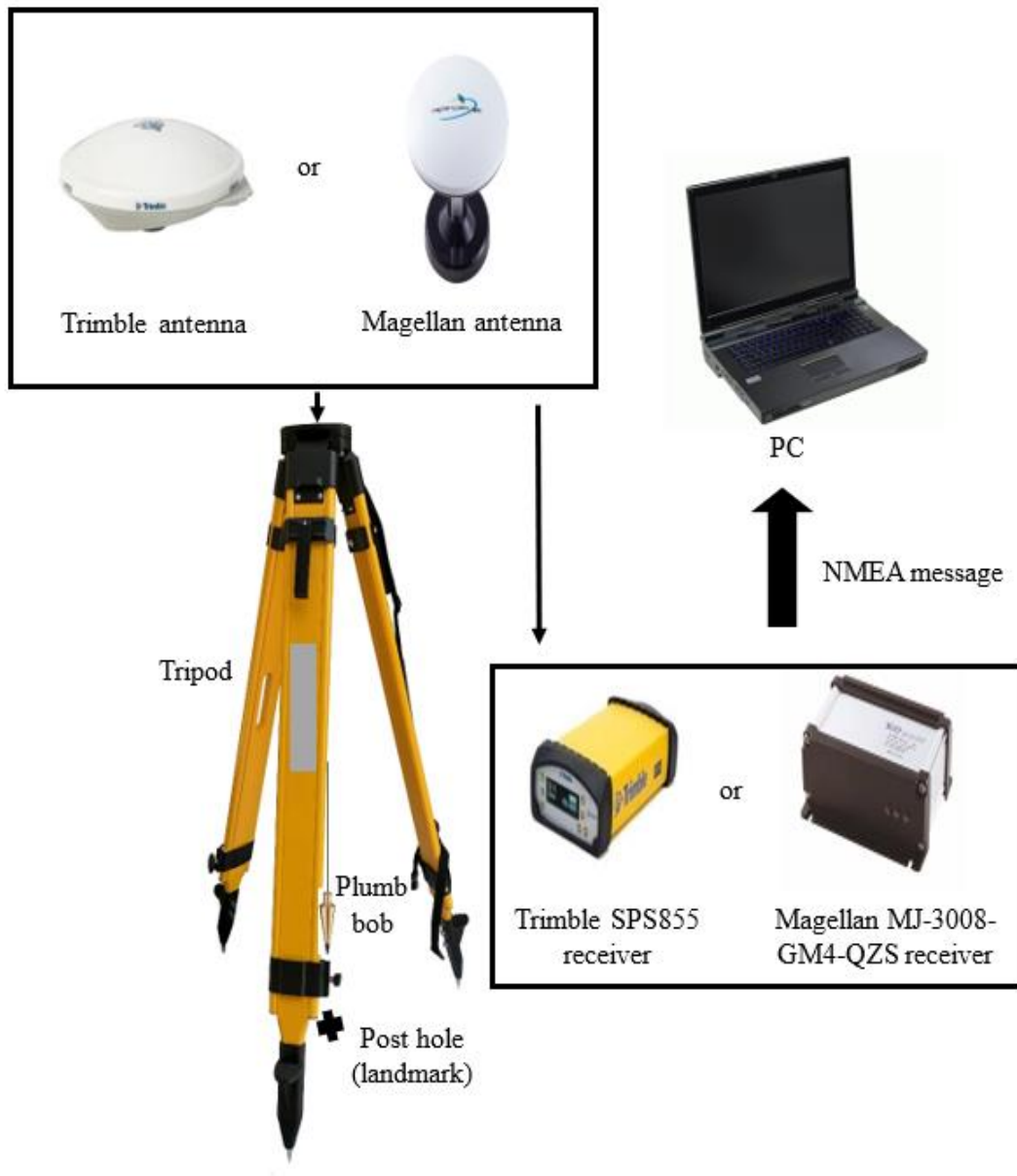
Figure 4.1 The setup of performance evaluation under static conditions.
