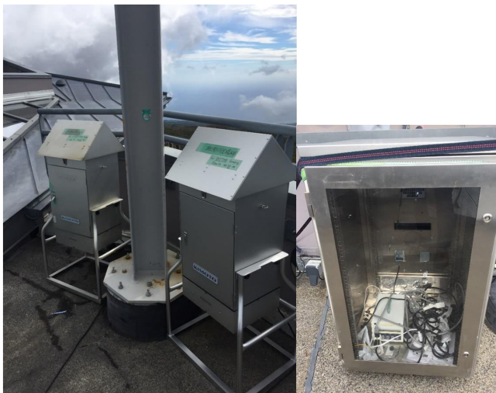
Figure 2.3 Two high-volume air samplers (HVAS; Model 120SL, Kimoto Electric, Osaka, Japan) in parallel located at the observatory (left). One sampler was used for the daytime sampling, and the other was used for the nighttime sampling. The power was supplied for each sampler automatically using a timer (right).
